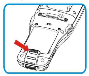
Figure 3: Remove main battery
