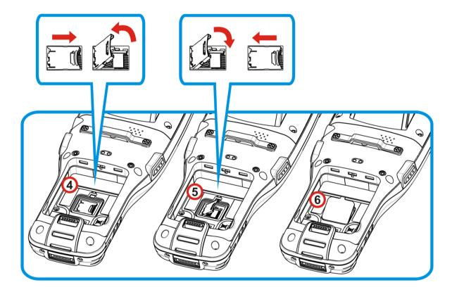
Figure 10: Inserting SD Card
