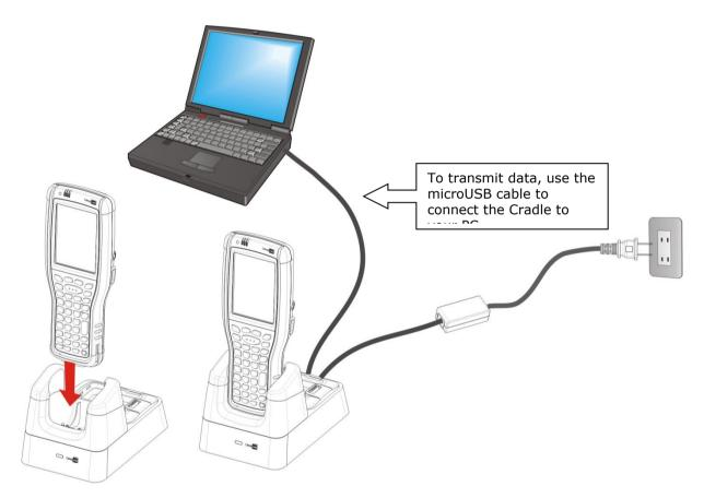
Figure 5: Direct Charging Using Cradle
