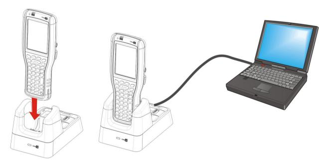
Figure 12: Direct Data Communication Using Cradle
