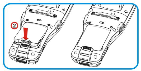
Figure 2: Install main battery
