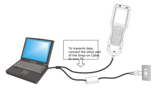
Figure 4: Direct Charging Using Snap-on Cable
