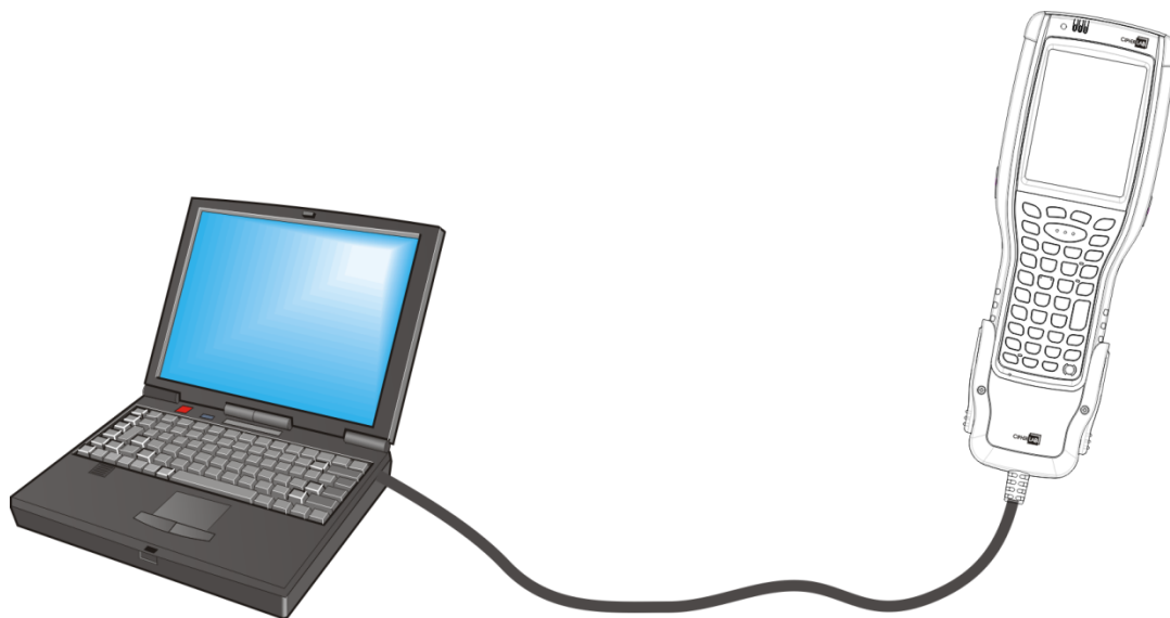
Figure 11: Direct Data Communication Using Snap-on Cable
