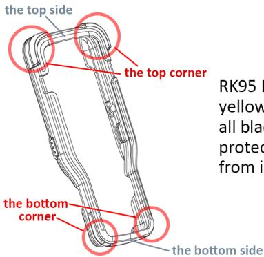
RK95 Rubber Boot, which is with the yellow frame in the front side while it is all black in the back side, is used for protecting the RK95 mobile computer from impact.
