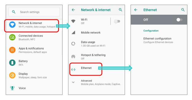
On "**Ethernet**" page, turn on the switch. Once the RK25 mobile computer is successfully connected to the Internet, the icon will displayed on the status bar.
