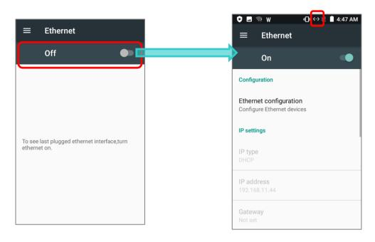
For further settings, please tap on "Ethernet configuration", and then tap "Manual" for Proxy and "Static" for IP Settings to expend the detailed settings. Please fill in the necessary fields base on your network environment.
