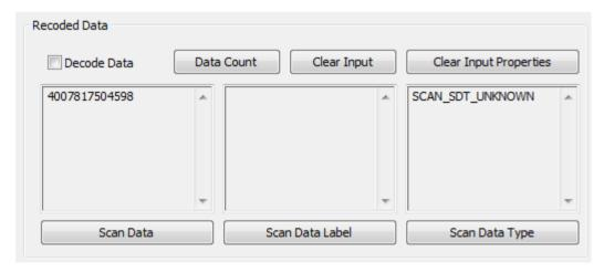
Note that the **Scan Data Label** text box display nothing and the **Scan Data Type** text box doesn't exactly show the data type information. You can tick the **Decode Data** checkbox to show the information.
