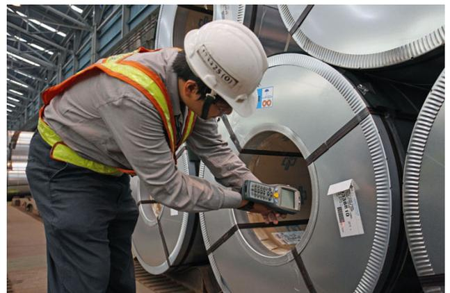
To scan bar codes on the stacked rolls while standing on the floor, 8500 mobile computers with extra-long-range lasers, which can read barcodes from over 13 meters, were chosen. Using the ergonomic pistol grip, workers use the 8500s for hours without fatigue. For warehouses storing smaller coils, CSC chose 8061 mobile computers for their handy pocket size and lower cost. With the deployment of the CipherLab 8061 and 8500 mobile computers, cycle counts are completed in half the time.
