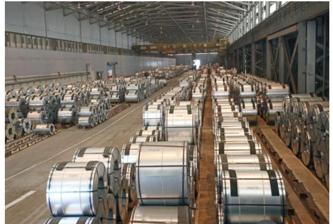
CSC sold 2.8 million tons of cold rolled coil steel in 2006, with an average weight of 14 tons. As coils leave the production line, bridge cranes carry them to assigned locations in the 300-meter long warehouse. Twice a month, a cycle count took three hours using four people in two teams with laptops. Both teams worked simultaneously, with one person obtaining product information and the other recording it on the laptop.
