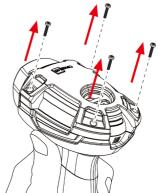
To remove the protective cover: Remove the screws to disassemble the protective cover.
