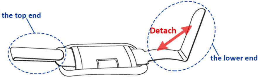
**Step 2:** Thread the velcro bands into the handstrap holes on the RK95 mobile computer, and then attach the velcro band.
