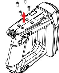
Slide the mount along the side slots until it is well fitted to the reader. Secure the mount with the included screws.
