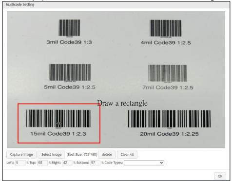
You can repeat the drawing process to make up to 10 rectangles. Each of them is labelled with a number. Enclosed in the rectangle any barcode types which the scanner is capable of decoding can be decoded.
