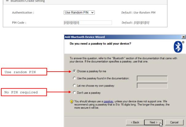
Note: When using Bluetooth HID, some device driver may not support pre-defined PIN code for authentication. In this case, make sure you disable the "Authentication" to have the scanner set to "No PIN or use random PIN" before pairing. While pairing, the host PIN code will be displayed on the computer screen. Have the scanner read the setup barcode "Enter PIN Code in Decimal" or "Enter PIN Code in Hexadecimal" to input the matching PIN code.
