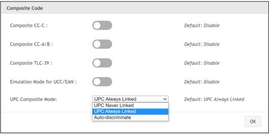
Enable the symbologies respectively so that the scanner can read Composite Code.
