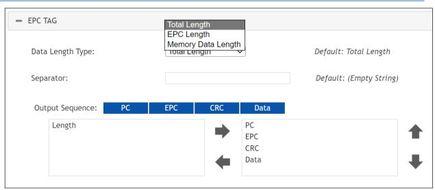
The EPC Tag section is divided into five fields as PC, EPC, CRC, Memory data, and Data Length. Separators can be specified between fields for clarity.
