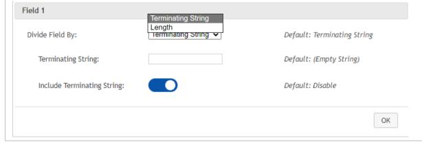
Data eligible for editing formats is divided into fields by user-specified rules – either using the field terminating string or specified field length.
