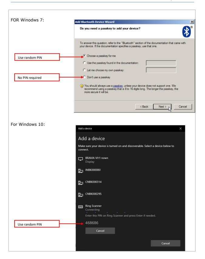
Note 1: When using Bluetooth HID, some device driver may not support pre-defined PIN code for authentication. In this case, make sure you disable the "Authentication" to have the scanner set to "Use random PIN (or No PIN)" before pairing. While pairing, the host PIN code will be displayed on the computer screen. Have the scanner read the setup barcode "Enter PIN Code in Decimal" or "Enter PIN Code in Hexadecimal" to input the matching PIN code.
