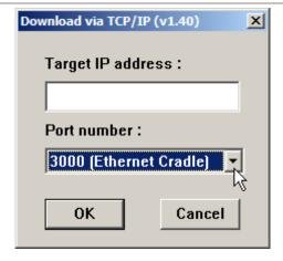
4) During downloading, the 1<sup>st</sup> LED (POWER) and 2<sup>nd</sup> LED (TX/RX) on the 8000/8300 Ethernet Cradle will be flashing by turns. Then, they will become solid red for approximately 3 seconds.
