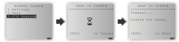
Warning: Before the download process is completed, do not disconnect the power to the cradle or remove the mobile computer from the cradle!
